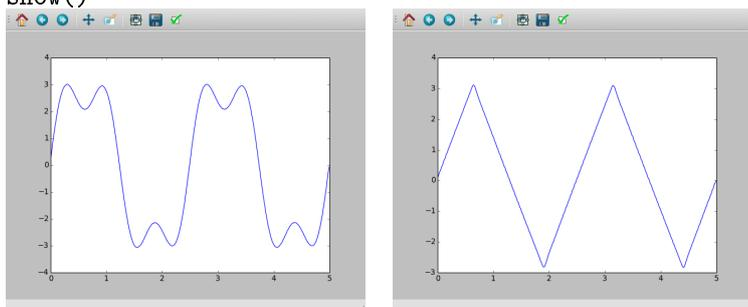
**load\_table(function, span)** The wave table can be loaded with a 512 element array. Connect WG to A1 and run the code below. After taking the absolute value, the table starts with 256, goes down to zero and then goes upto 255, tracing a triangular wave. The table output also is shown above.
