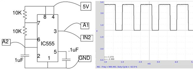
Circuit is shown in figure. The frequency is given by  $f = 1 / (\ln 2 \times C \times (R_1 + 2R_2))$ . The HIGH time is given by  $\ln 2 \times C \times (R_1 + R_2)$  and LOW time by  $\ln 2 \times C \times R_2$ .
