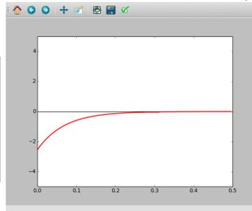
In an RL circuit  $V = IR + L \frac{dI}{dt}$  and solving this will give  $I = I_0 e^{-\frac{R}{L}t}$ . The coefficient of the exponential term  $R/L$  can be extracted from the graph of voltage across the inductor. The resistance of the inductor coil should be included in the calculations,  $R = R_{ext} + R_L$ .
