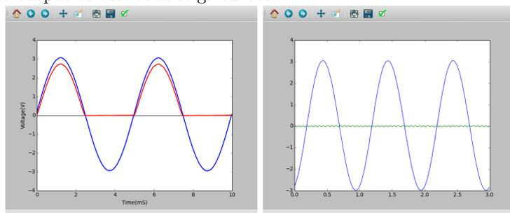
**capture4(Number of samples, time interval)** Digitizes the inputs A1,A2,A3 and MIC together. The number of samples could be upto 10000. The time gap between two consecutive samples is given in microseconds (range 2 to 1000 usec).
