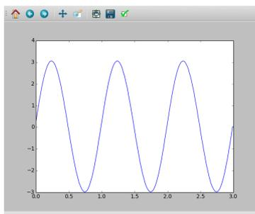
**capture2(Number of samples, time interval)** Digitizes the inputs A1 and A2 together. The number of samples could be upto 10000. The time gap between two consecutive samples is given in microseconds (range 2 to 1000 usec).
