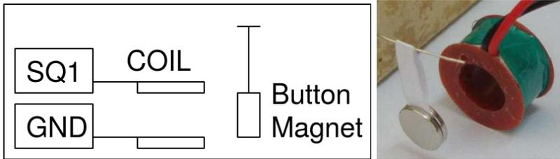
**Procedure** Make a pendulum using two button magnets and a piece of paper. Suspend it and place the 3000T coil near that, as shown in figure.
