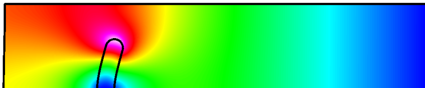
Figure 11.4: Displacement distribution of the obstacle in channel case.
