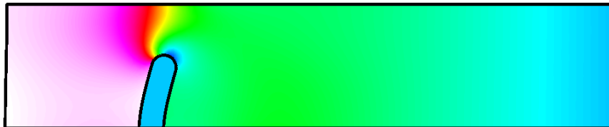
Figure 11.3: Pressure distribution of the obstacle in channel case.
